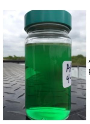
APS; chemical injected into pipeline to remove paraffin
