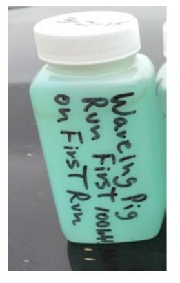
Brand X chemical injected into pipeline to remove paraffin
