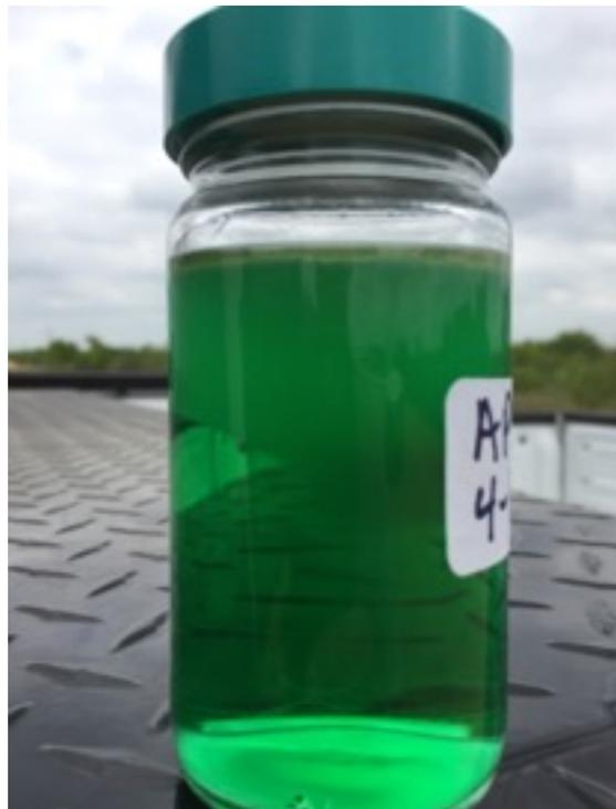
APS; chemical injected into pipeline to remove paraffin
