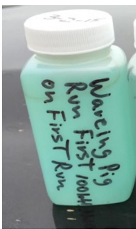
Brand X chemical injected into pipeline to remove paraffin
